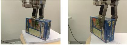
Fig. 7: Illustration of the grasps executed by the robot. The left image shows a “middle” grasp, which always succeeded, while the right image shows an “extremity” grasp which always failed. The object was continuously explored between these two points.
