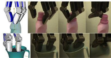
Fig. 3. Grasps that are stable in simulation but failed in real experiments.
