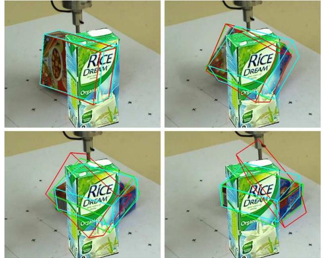
Fig. 8. The toughest case: toppling combined with occlusion. (colour-based tracking with prediction: green, without prediction: red, pure prediction: blue)
