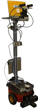
(a) The Dora platform: a P3 mobile robot base with a custom-built super-structure and different sensors.
